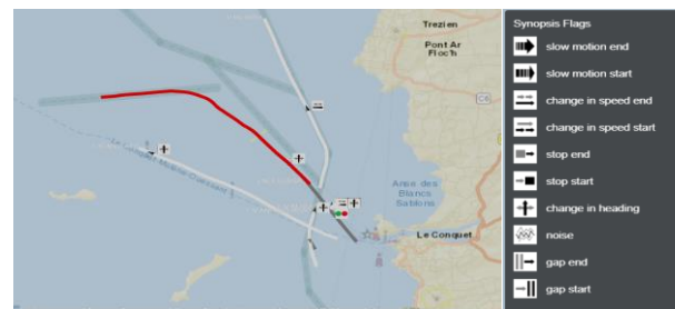
Figure 2: Interactive visual exploration of raw (red) vs. predicted (grey) location data in IVA (online) tool, along generated synopses (icons).
